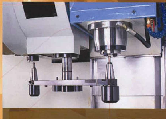
■ Cam operated tool changer, high speed tool change (2.5 secs, tool to tool at 60 Hz) (Optional)
